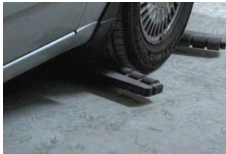
Bước 2: Cánh tay robot nâng xe (Step 2: Robot arms lift car up)
